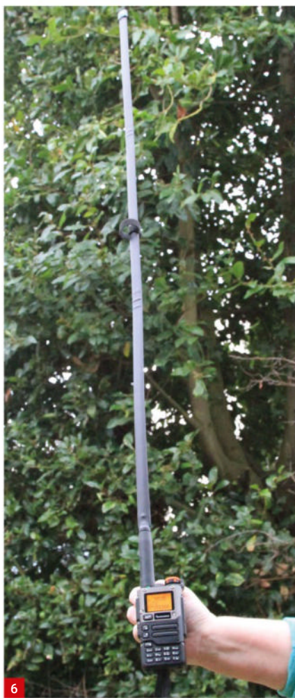
Fig. 5: The Abbree sitting on Quansheng folded over. Fig. 6: The Abbree extended to full length.
