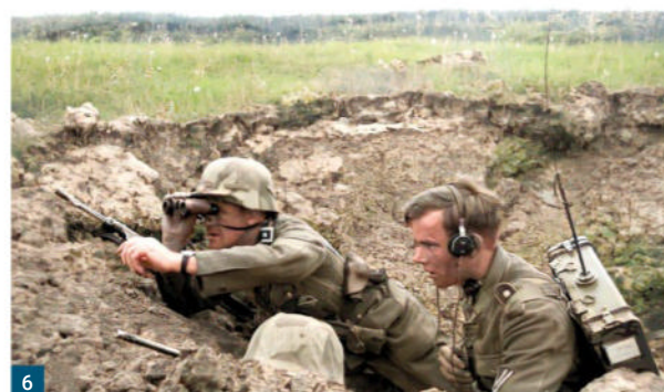
Fig. 2: Operational setup of the Torn.Fu.d.2 VHF Transceiver. On the right is the Zubehör (Accessories Box), which housed the batteries, seen here plugged-in. The vertical six-rod antenna could extend to 1.8m. ( funksammlermilitaria.com )
