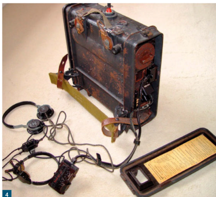
Fig. 1: The Torn.Fu.d.2 VHF (dual Morse and voice) transceiver became the standard portable radio set used by the infantry of the Wehrmacht and Waffen SS at regimental, battalion and company levels. ( laud.no/ww2 )
